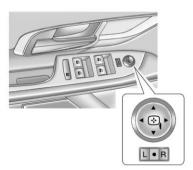
Controls for the outside power mirrors are on the driver door.
